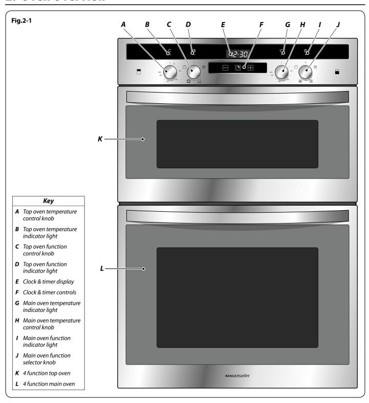
The oven (Fig.2-1) has two multi-function oven cavities with four retractable push-in controls. The left-hand knobs control the top oven and right-hand knobs control the main (bottom) oven function and temperature operation. There is also a touch sensitive timer.
